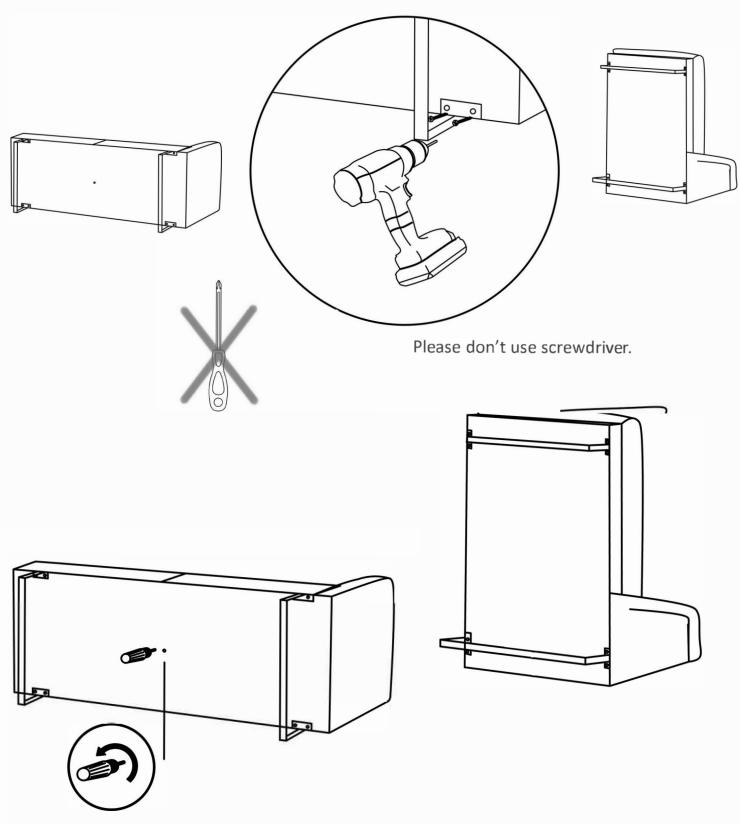
After finishing the assembly of the iron legs, let's connect the middle legs.
